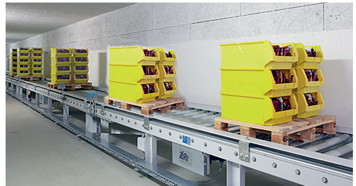
Fully automated conveyor belt running between warehouse and manufacturing site
