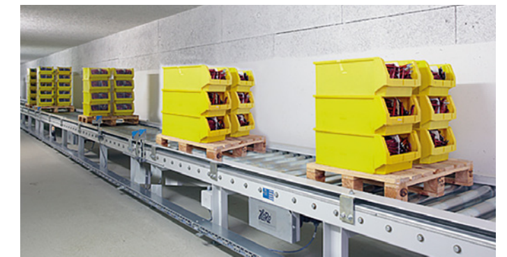
Fully automated conveyor belt between warehouse and production
