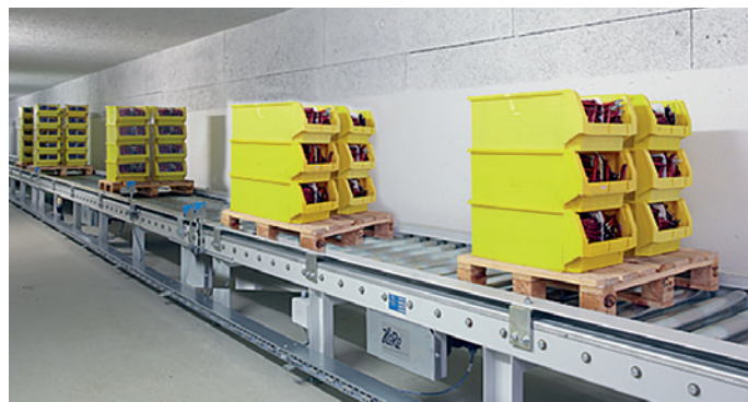
Fully automated conveyor belt running between warehouse and manufacturing site
